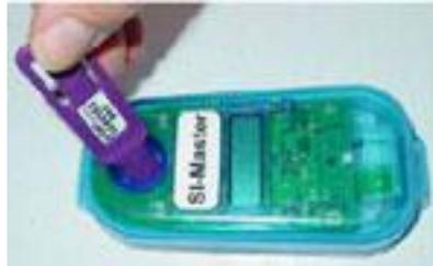
2. Press the coupler rod into the SI-Master so that friction holds it in place.
